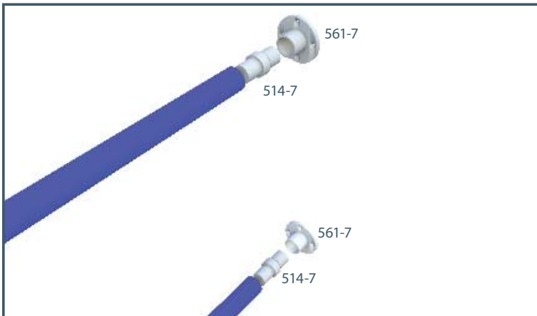
HANDRAIL RAILING END: Mount the 561-7 to the wall. The handrail or mid-rail tube is then connected to this fitting using a 514-7.
