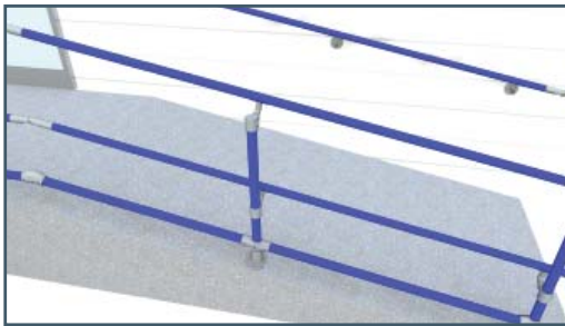
A) HANDRAIL: Handrail must be a continuous smooth surface. Handrail must be on both sides of ramp or stairs.
